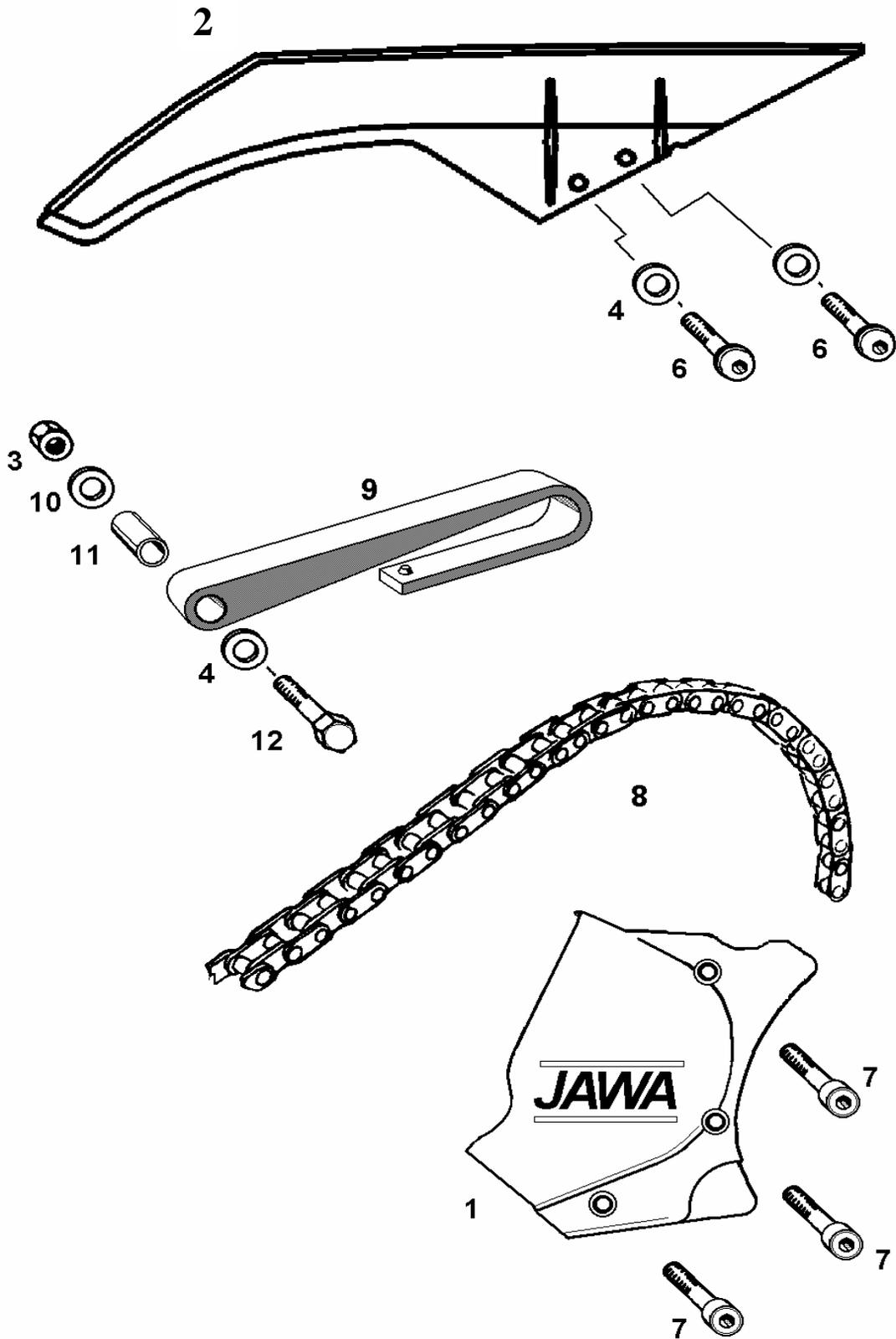
**03****KRYT ŘETĚZU - KETTENVERKLEIDUNG - CHAIN COVER - COUVRE CHAÎNE****650 cm<sup>3</sup>
